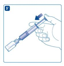
Click the vial adapter, still attached to the syringe onto the powder vial. Hold the syringe slightly tilted with the vial facing downwards. Push the plunger slowly to inject the solvent into the powder vial. Make sure not to aim the stream of solvent directly at the powder as this will cause foaming.
